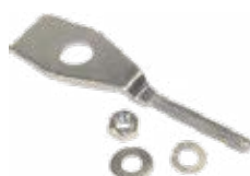
REF: 101401 TENSOR CADENA AK 110 HONDA C100 BIZ DIAM 12.5mm
