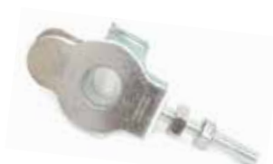
REF: 101592 TENSOR CADENA DER-IZQ YAMAHA FZ16-FAZER 150- FZ2.0 FRENO DE BANDA-FZS 150 FI
